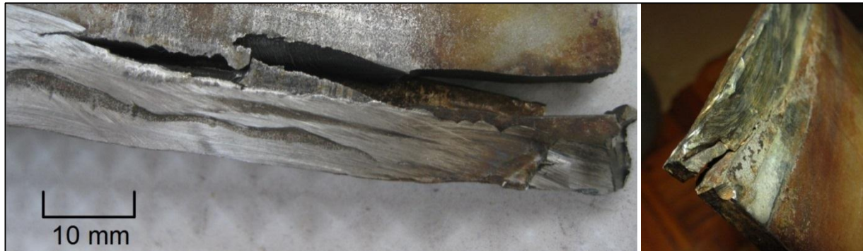
Figure 4 – Representation of two of the cracks found at the embedded regions of the removed blades.
