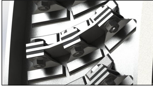
Figure 14 – Detail of the embedded region of the design suggestion for a new stator. Note the intermediate material between the blade and the supports, which can be made from absorbing materials to modify the dynamic response of the blade.
