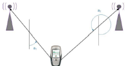
Figure 2.11: A simple illustration of the Angle of Arrival technique.
