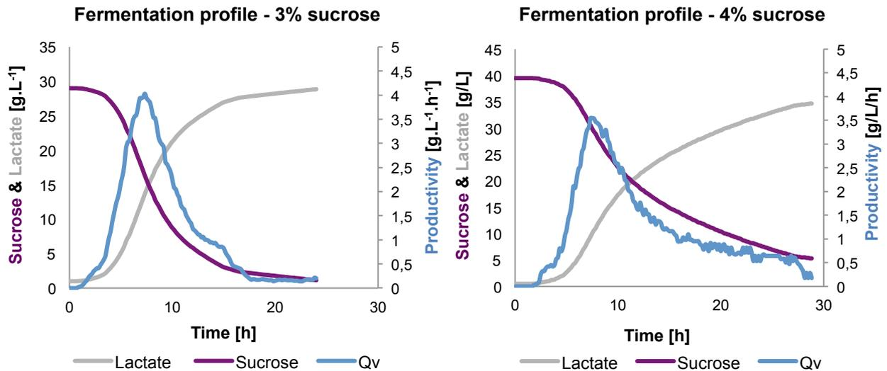
**Figure 1.2, 1.3** - Average of the fermentation profiles of all experiments performed with the standard conditions with 3% and 4% of sucrose, respectively.
