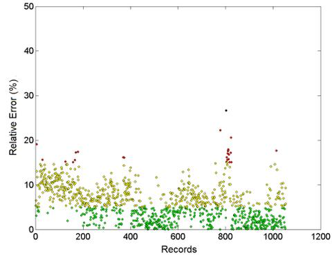
Figure 6: Difference between modelled and real PV power for irradiance in  $[350; 500] W/m^2$ .
