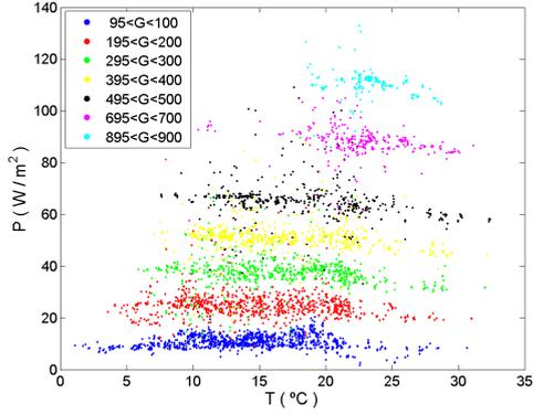
Figure 3: PV power Vs Temperature.
