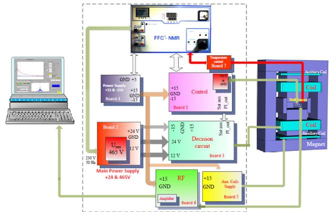
Figure 3: Architecture of a modern fast field cycling relaxometer (proposed by Roque et al [10]).
