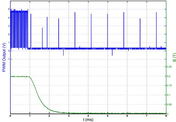
Figure 11: Magnetic field strength and PWM waveform during a downward transition.
