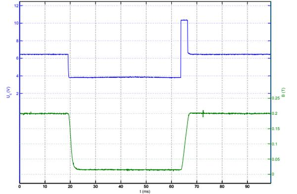
Figure 12: IGBT gate voltage and  $B_0$  in a complete field cycle.
