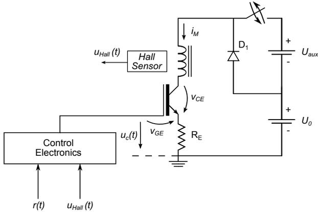
Figure 7: Main power supply control circuit of the FFC relaxometer.
