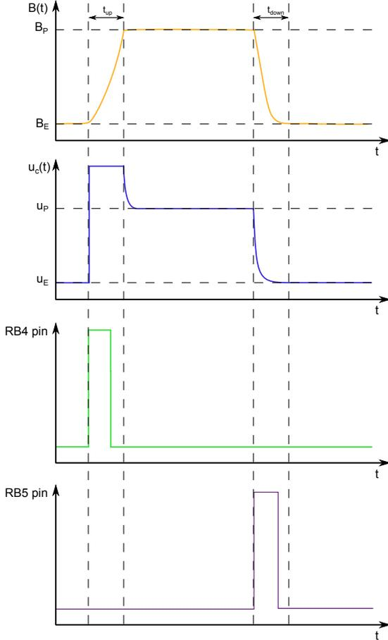
Figure 9: Field cycling sequence. Shown are the magnetic flux density  $B(t)$ , the IGBT gate voltage  $u_c(t)$  and the states on RB4 and RB5 pins.
