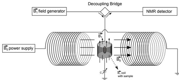
Figure 2: Block diagram of a typical configuration of a NMR spectrometer.
