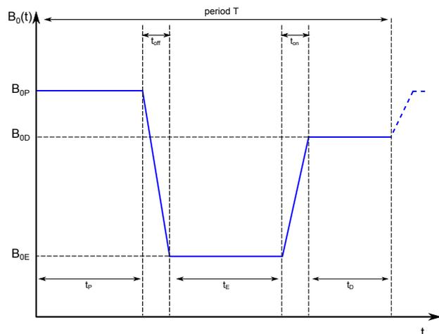
Figure 1: Time diagram of the FFC-NMR spectroscopy technique.
