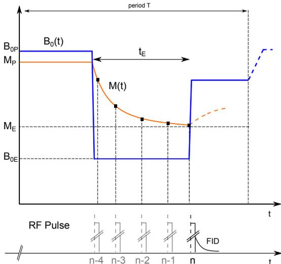
Figure 6: *Zeeman* field cycle with the representation of the measurements for different lengths of  $t_E$ .
