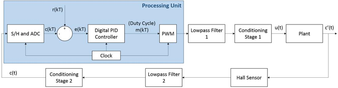
Figure 10: Conceptual scheme simplified of the control system implemented.
