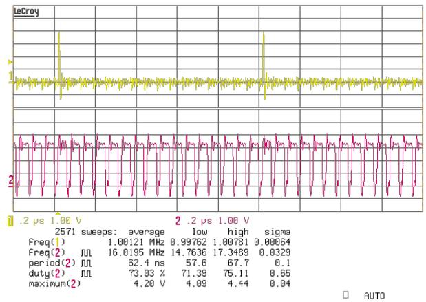
Fig. 14 - Oscillator and pulse generator output.
