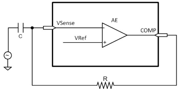
Fig. 20 - Schematic of the error amplifier test circuit.
