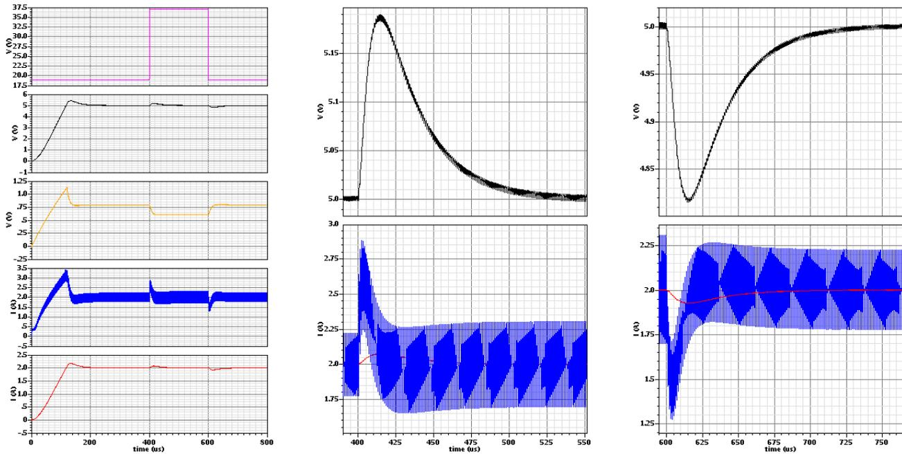
Fig. 10 - Input voltage step response of the proposed converter.
