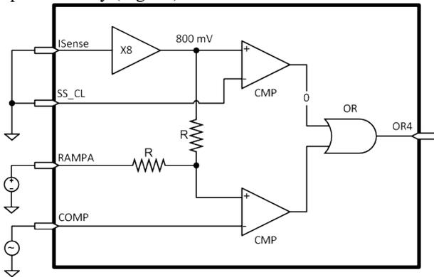
Fig. 16- Schematic of the circuit used to test the comparator.
