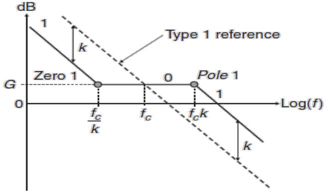
Fig. 4 - Type 2 compensator bode plot [7].
