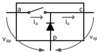
Fig. 2 - PWM Switch model, a is the active port, p is the passive port and c is the common port [7].
