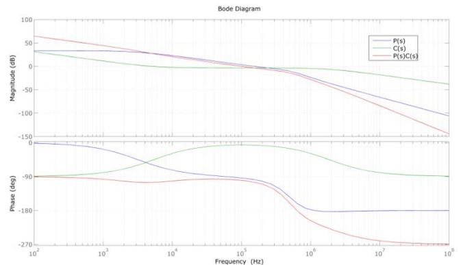
Fig. 8 - Bode plots, red line - closed loop, green line - compensator and blue line - open loop.
