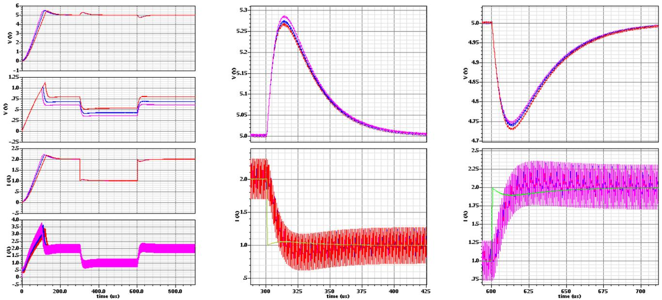
Fig. 9 - Load step response of the proposed converter for the three different input voltage
