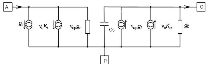
Fig. 3 – PWM switch small signal model for current-mode control [7].
