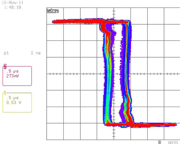
Fig. 15 - Under Voltage Lockout hysteretic output.
