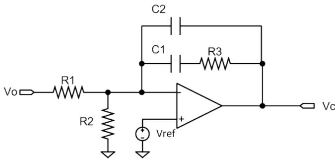
Fig. 5 - Compensator circuit diagram.
