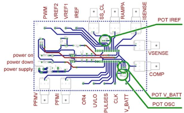
Fig. 13 - Test board to do the "Test On A Chip".
