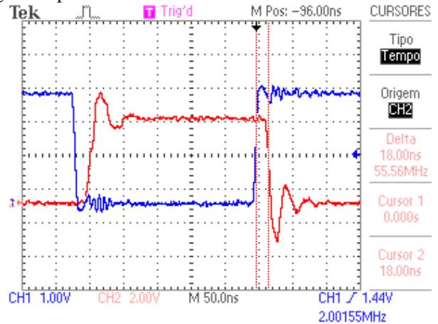
Fig. 18 - Non-Overlapping and Power Stage output.
