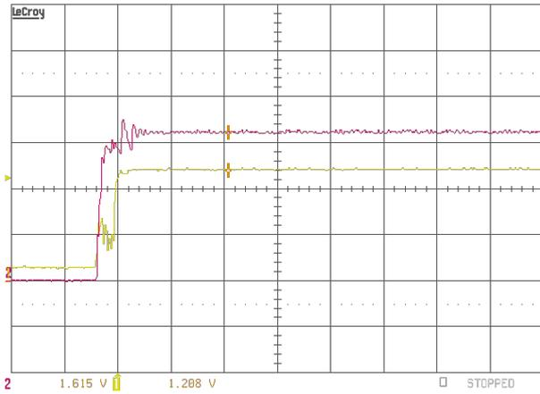
Fig. 19 – Transient response of band gap voltage reference.
