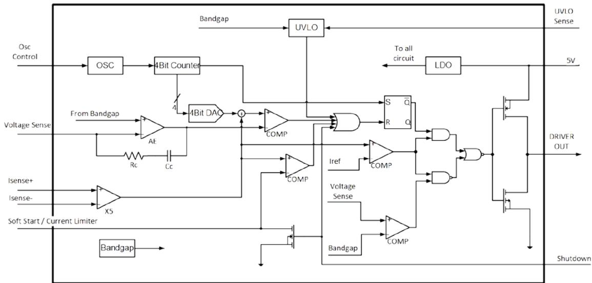
Fig. 7 - Topology of the control circuit.
