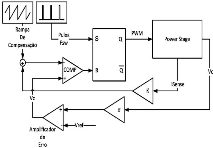
Fig. 1 - Current mode control scheme.
