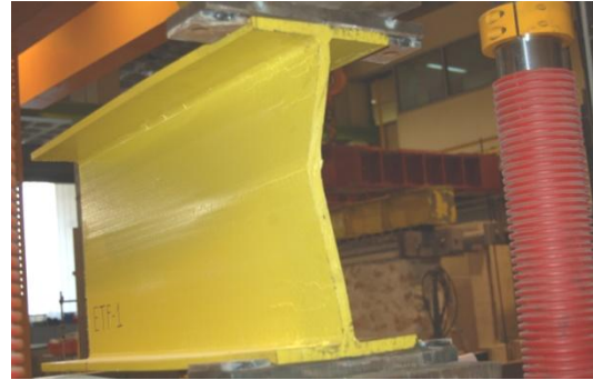
Fig. 4: Test specimen I400-ETF-100-1: Buckling of the web.
