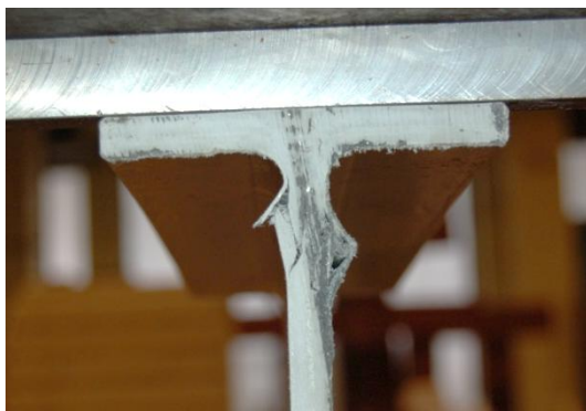
Fig. 1: Test specimen I200-ETF-15-2: Rupture near the web-flange junction.
