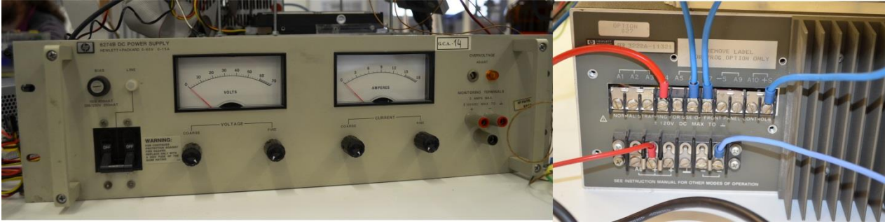
Figure 5.6 – Hewlett Packard 6274B DC Power Supply and Rear-Panel connections
