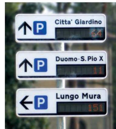
Figure 3.6 - VMS informing in real-time the availability of parking. Source: (Smart Parking Systems: "Intelligent management of the parking area")
