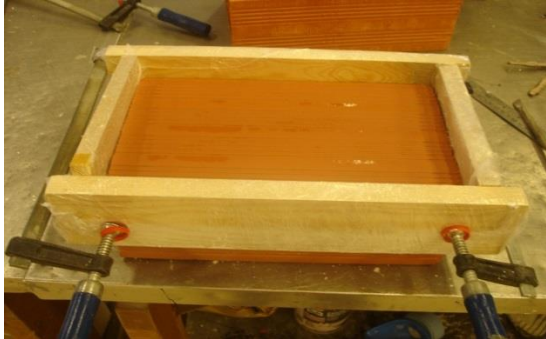
Figura 3.21 – Cofragens de madeira
