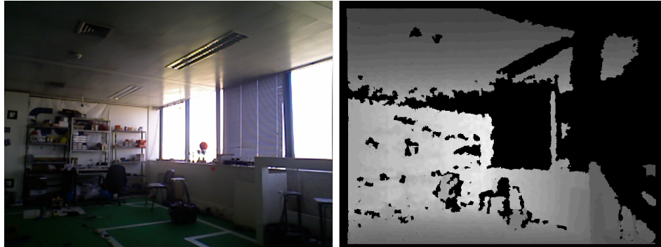
Figure 3.2: RGB-D Image from the Xtion Pro
