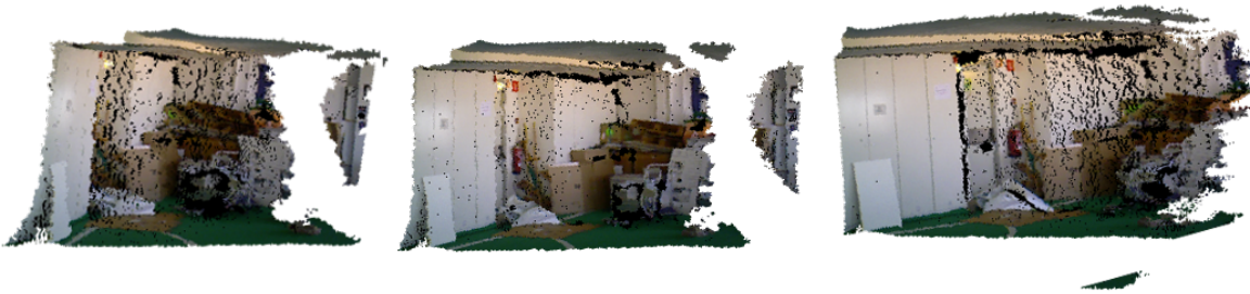
Figure 2.5: One RGB-D pointcloud captured with a Asus-Xtion Pro. Views of the same cloud from different perspectives
