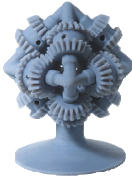
Fig. 1: Example of printed object using the three-dimensional modelling. Due to its complexity, it is not possible to manually creating it as a single piece. (Source: Proto3000.com (2013))
