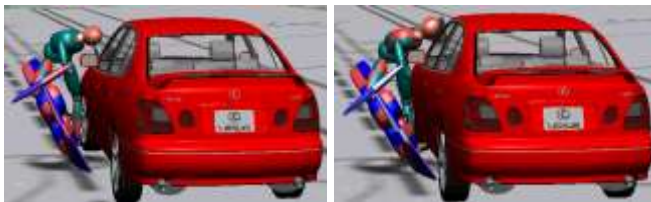
Figures 3.10 and 3.11 - New simulation sequence of the accident with head contact in initial impact.
