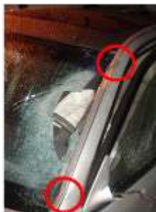
Figure 3.12 - Broken windshield on the left and impact dents (red circles) on the left a pillar.
