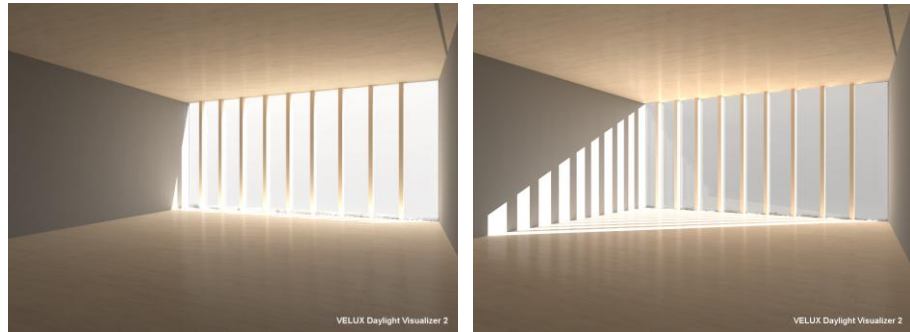
Fig. 93 Classroom on the ground floor at noon on the 21st of June (on the left) and on the 21st of December (on the right)
