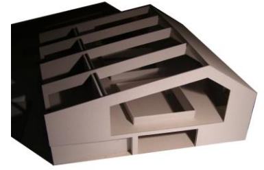
Fig. 84 Section of the children's area; structure that supports the roof
