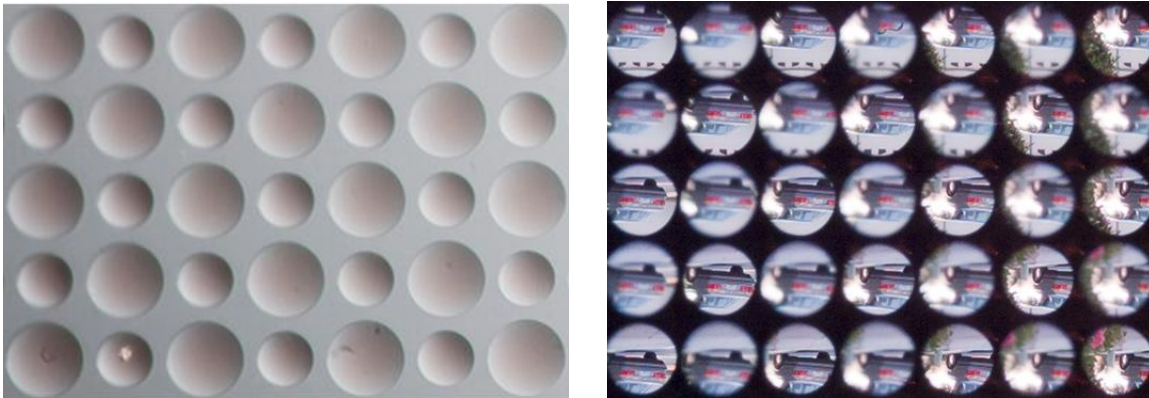
Figure 2.19 – Left) MLA with micro-lens of different focal lengths, which are coupled with the diameter of each micro-lens; Right) Array of micro-images captured with the MLA on the left; notice the differently focused micro-images, interleaved accordingly.
