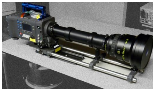
Figure 2.20 - ARRI Alexa camera fitted with the ARRI holographic capture tube [15].
