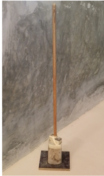
Figure 3: Compactor of the 1 st trial embankment.
