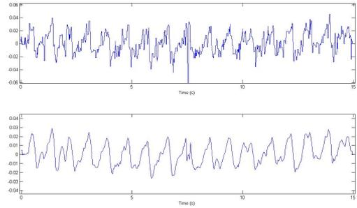
**Figure 4:** Top: IR signal before filtering. Bottom: IR signal after mean filter application.
