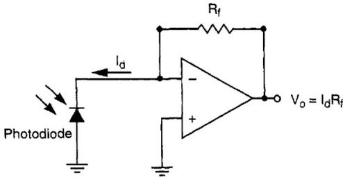
**Figure 2:** Transimpedance Amplifier Circuit Diagram [4].
