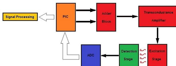
**Figure 1:** Block Diagram of the Prototype. The black arrows represent analog signal, the white arrows represent digital signal and the red arrows are light photons.
