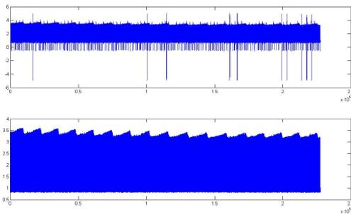
**Figure 3:** Top: signal before filtering. Bottom: signal after median filter application.
