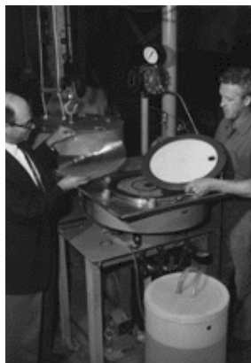
Figure 2.1 - Professor Sidney Loeb and engineer Ed Selover remove newly manufactured reverse osmosis membrane from plate-and-frame production unit [21].
