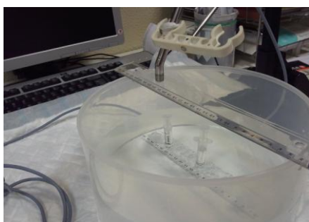
Figure 1 – Position of the ^{99\text{m}}\text{Tc} sources in a phantom composed of the polypropylene container.
