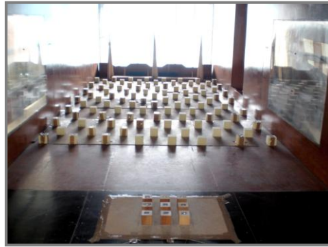
Figure 3 - Roughness elements used on atmospheric boundary layer simulation.
