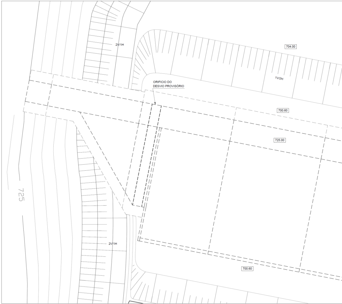
Figure 7 - River diversion; Orifice on dam body. Plan.
