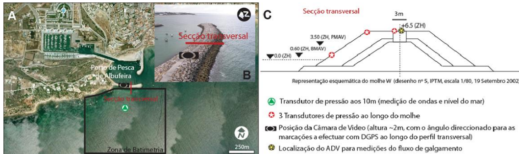
Fig.2. (A) Aerial Image of Albufeira's Fishing Harbor (adapted from Google Earth, 2006) showing the zone where the works will be performed of bathymetry, video camera's location and pressure transducer to ~10m depth; (B) West breakwater of Albufeira's Fishing Harbor where will be performed the field campaigns with section in study indicated; (C) Schematic representation of the breakwater section and equipment positioning (PTs e ADV) [19].
