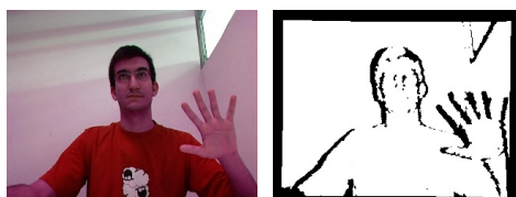
Figure 4.7: Simple video frame captured with the RGB camera (left); Depth map of the environment (right).
