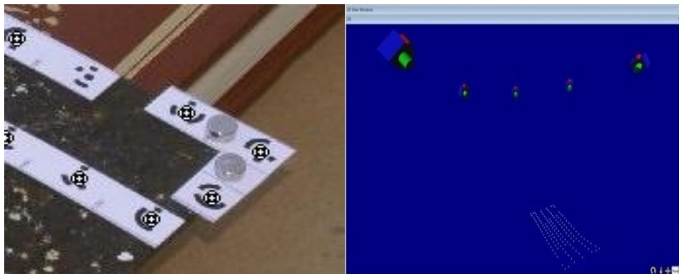
Figure 7.5. Left: Target point in the corner. Right: Cloud of points' 3D model.
