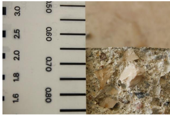
Figure 20 – Impregnated depth on a specimen in concrete B2 with the product A applied
