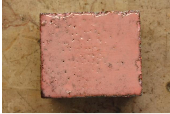
Figure 1 – Appearance of a sample in concrete B1 after the application of product B mixed with the pigment
