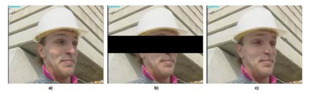
Figure 11 - Inter-frame prediction a) original b) losses detected c) prediction
