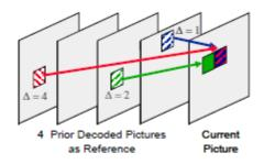
Figure 5 - Multiple reference frame motion compensation
