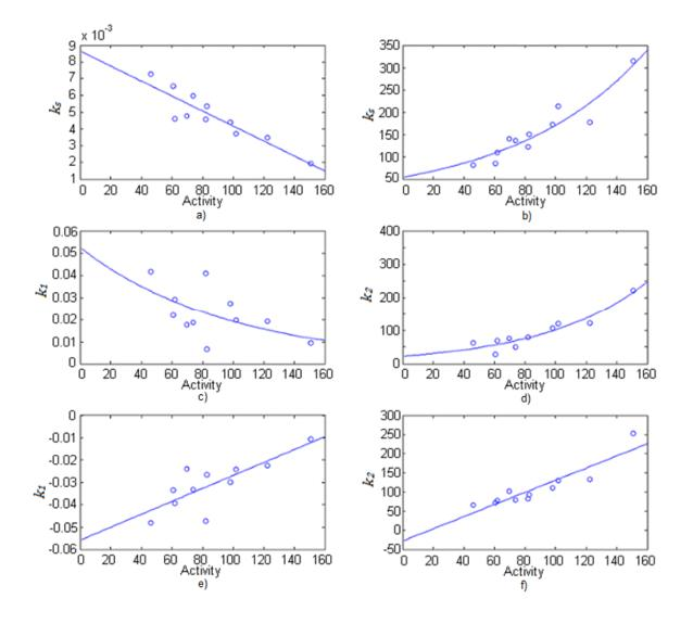
Figure 21 - Model parameters versus estimated video activity, and resulting regression curves, for: a) linear model, b) exponential mode, c) and d) sigmoid1 model, e) and f) sigmoid2 model, using the estimated MSE and video activity values
