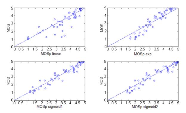
Figure 22 - MOSp versus MOS for the four prediction models using true MSE and true activity
