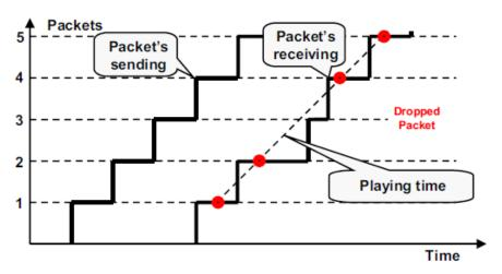
Figure 7 - Packet loss due to delay
