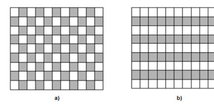
Figure 9 - FMO a) checker-board mode b) interleaving mode
