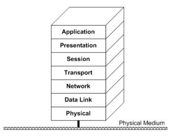
Figure 6 - The OSI reference model
