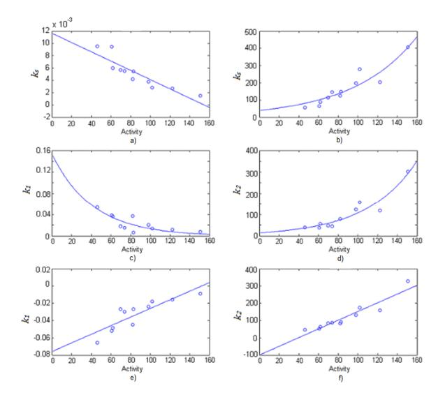
Figure 20 - Model parameters versus video activity, and resulting regression curves, for: a) linear model, b) exponential model, c) and d) sigmoid1 model, e) and f) sigmoid2 model, using the true MSE and video activity values.
