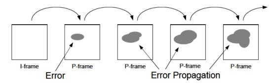
Figure 8 - Error propagation from a single error
