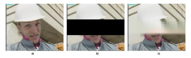
Figure 10 - Intra-frame prediction a) original b) losses detected c) prediction
