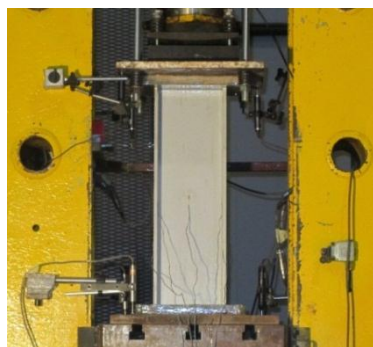
Figure 12 – Short column test setup for column C5
