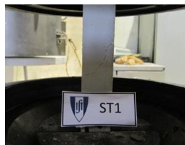
Figure 10 – 10° off-axis tension coupon test failure mode.
