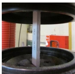
Figure 6 – Tension coupon test failure mode.
