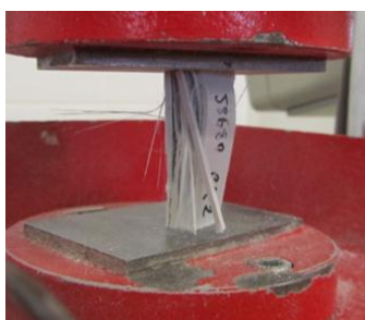
Figure 5 – Compression coupon test failure mode.
