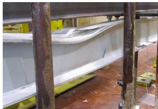
Figure 32 – Four-point bending beam buckled configuration after collapsing.
