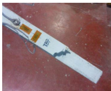
Figure 9 – Tension coupon test failure mode to obtain Poisson's ratio.
