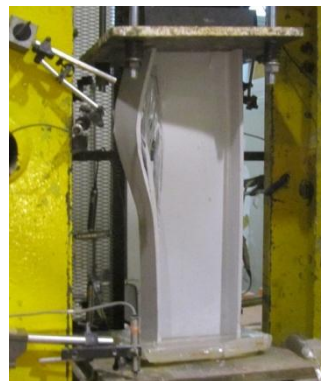
Figure 16 – Column C3 buckled configuration after collapsing.
