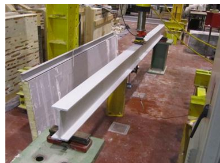
Figure 20 –Three-point bending beam test setup.
