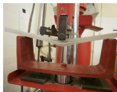
Figure 7 – Three-point bending coupon test failure mode.
