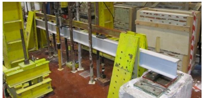
Figure 24 – Four-point bending beam test setup.
