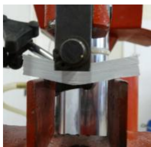
Figure 8 – Interlaminar coupon test failure mode.
