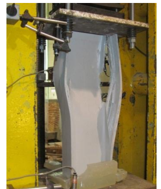
Figure 17 – Column C5 buckled configuration after collapsing.
