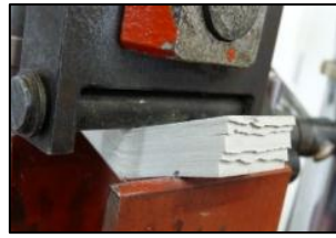
Figure 3. Interlaminar shear test failure
