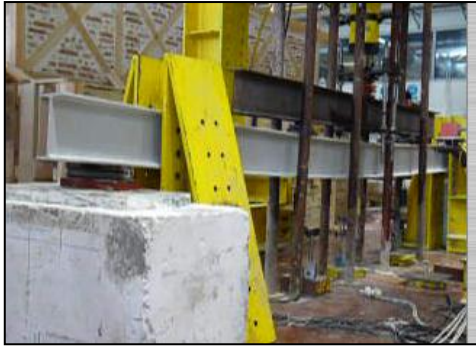
Figure 26. Global transverse deflection on the brink of collapse
