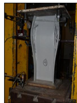
Figure 12. Failure mode with tearing of flanges from the web
