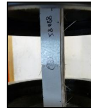
Figure 5. Tensile test failure
