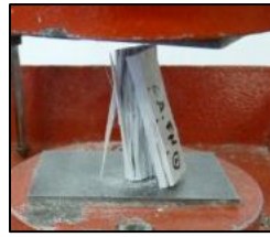
Figure 4. Compressive test failure
