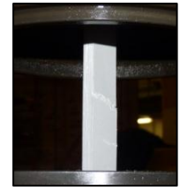
Figure 6. In-plane shear failure
