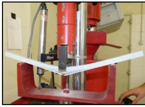
Figure 2. Bending test failure
