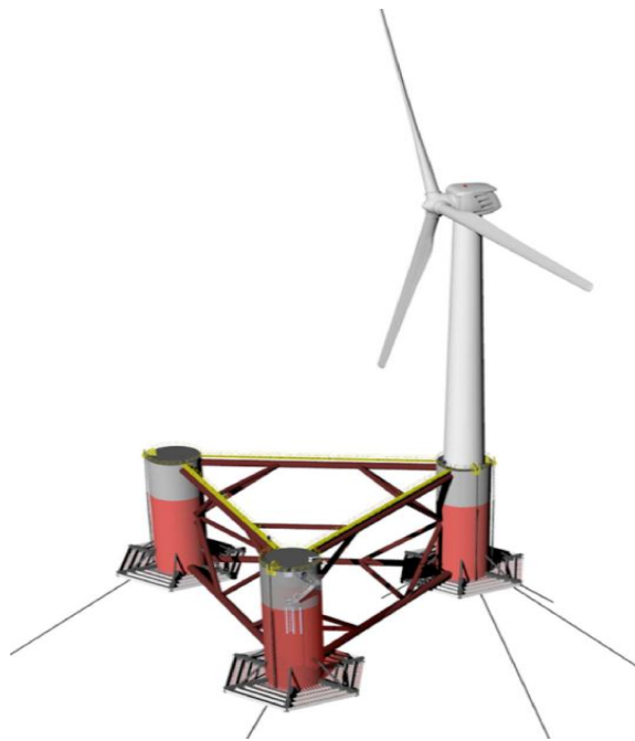
Figure 2.4: Semi-submersible type floating wind turbine
