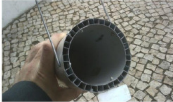
Figure 4.21: Double wall exhaust duct.
