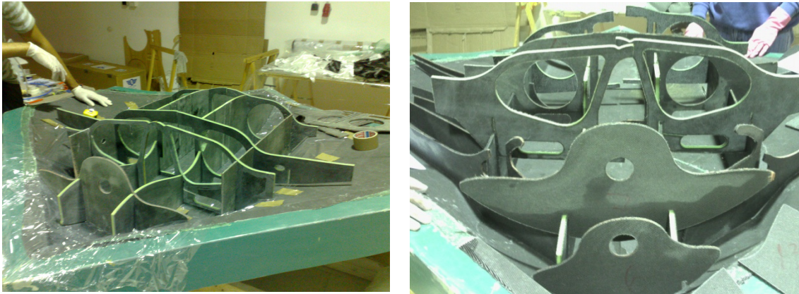
Figure 4.23: Central bulkheads assembly.
