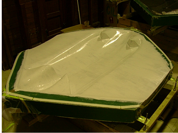
Figure 4.10: Mould covered with gel coat.
