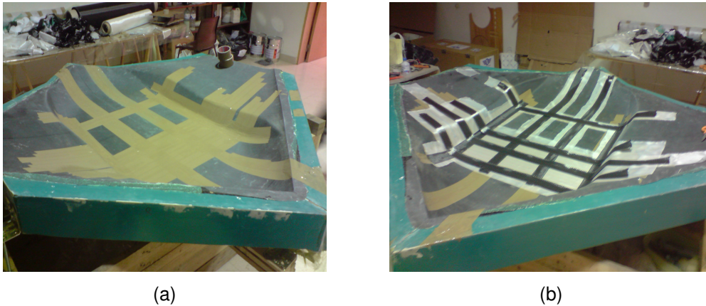
Figure 4.37: Skin-bulkheads joint: (a) Preparation of the mould; (b) View of the fibercarbon sheet.
