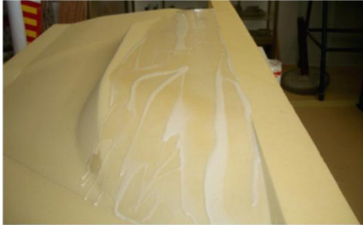
Figure 3.4: Micro slurry application.
