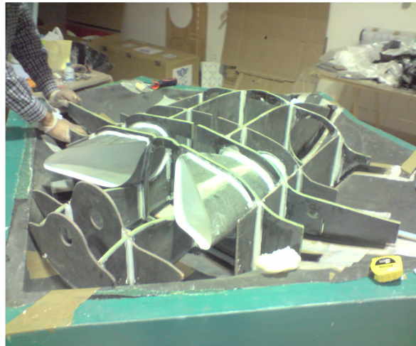
Figure 4.28: Glue of the forward bulkheads.
