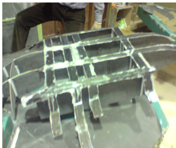
Figure 4.40: Sheets glued to the structure.
