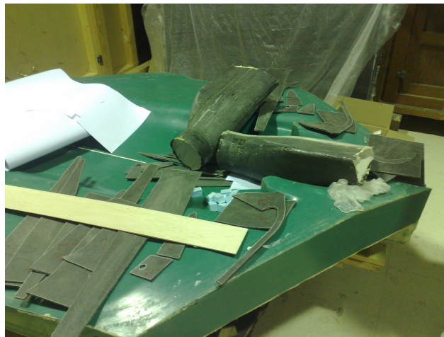
Figure 4.22: Bulkheads and air ducts.
