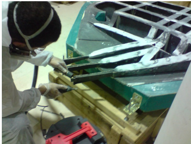
Figure 4.35: Cutting the carbon sheet and the plywood.
