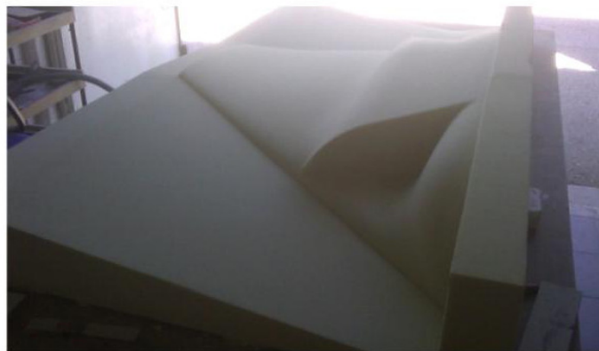
Figure 3.3: Plug after sanding.
