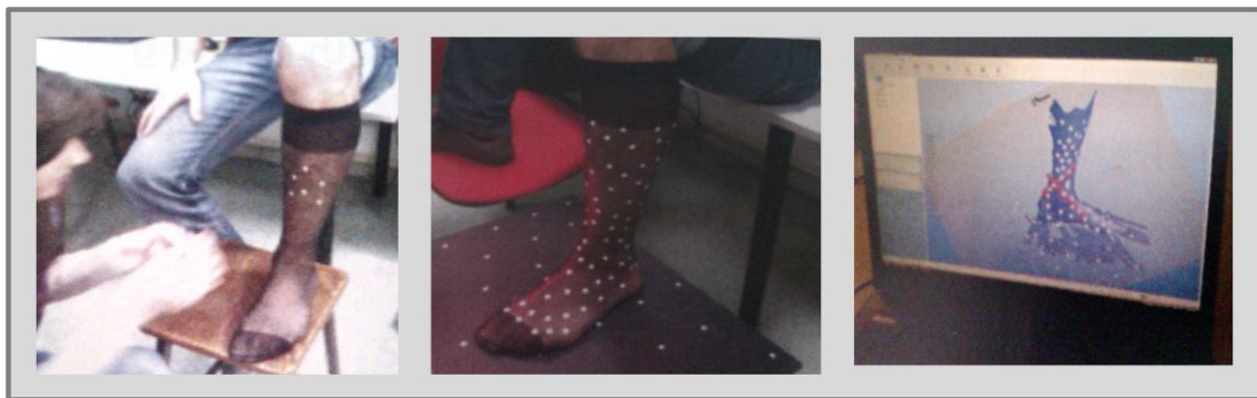
Figure 5. 1 - Left: First step on the 3D scanning, marking the reference points for the points cloud creation; Middle: Reference points marked. Lower limb prepared to be scanned; Right: Points cloud generated after the 3D scanning. This technique often introduces some points that are not part of the scanned object, so the points cloud needs to be edited (Ana Luisa, 2010).
