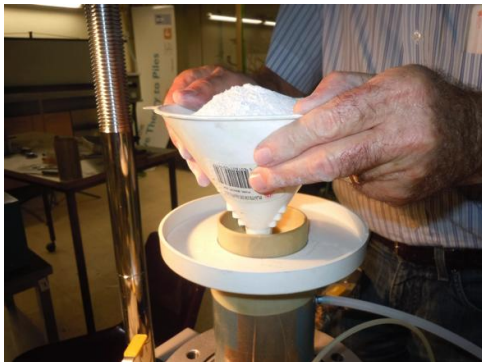
Figure 3.2 – Dry funnel deposition of the Silty Sand specimens
