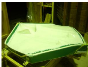
Figure 4.3: Mould covered with gel coat.
