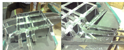
Figure 4.12: Sheets glued to the structure.
