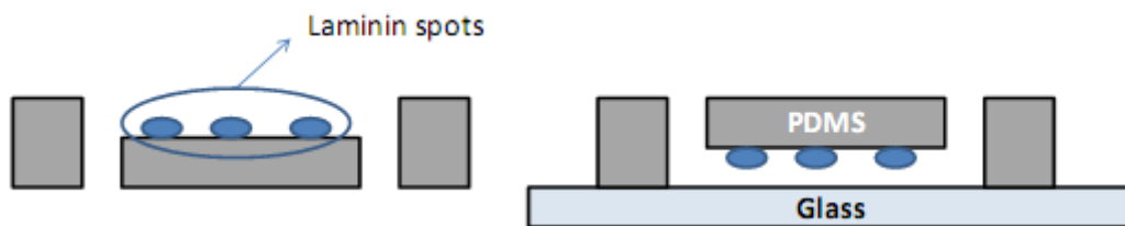
Figure 46. Illustration of the microdevice used in initial microfluidic experiments. Laminin was directly spotted inside the microchannel, which was then sealed with a glass slide.
