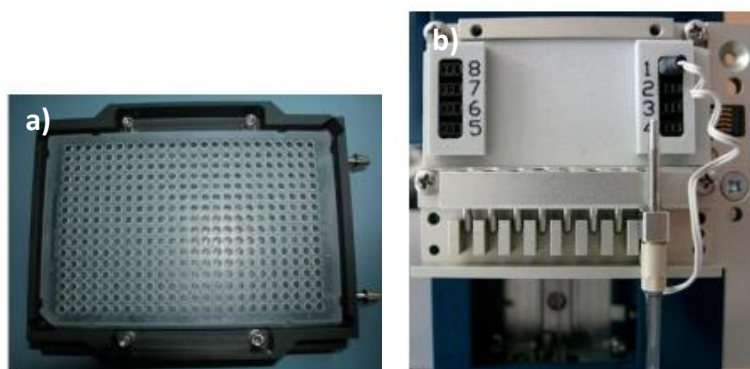
Figure 24. a) 96-well plate contained within the Nanoplotter basic device. b) Nanoplotter tip holder.
