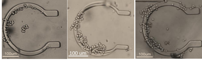
Figure 52. Microarray of PDMS traps inside the microchannel. Using a cellular concentration of 3 \times 10^6 cells/ml, less cells were immobilized inside the PDMS traps, compared with Figure 51-d). The fluid flowed from right to left.
