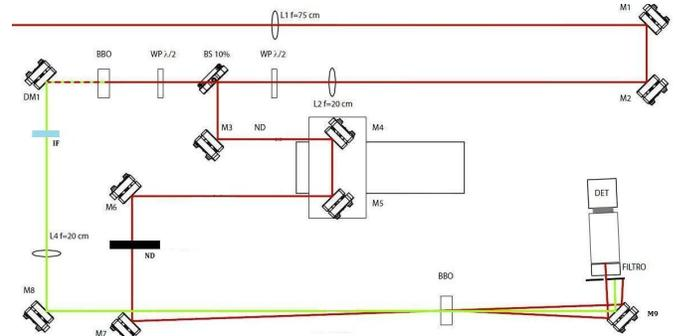
Figure 2: Layout of OPAC. L1-L4: lenses, M1-M8: mirrors, WP: waveplates, BBO: BBO nonlinear crystal, DM: dichroic mirror, ND: set of calibrated neutral density filters, DET: photodiode detector, IF: infra-red filter.
