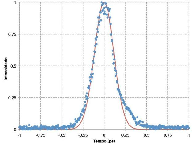
Figure 4: Measured third-order autocorrelation (blue dots) and Gaussian fit (red line).
