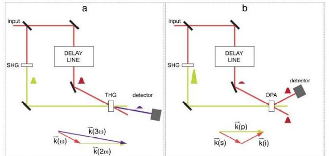
Figure 1: Schematic of (a) third-order autocorrelator and (b) optical parametric amplifier correlator. SHG/THG: second/third harmonic generation crystals, OPA: optical parametric amplification crystal. Also shown are the corresponding wavevector geometries, in the first case involving the fundamental, 2<sup>nd</sup> and 3<sup>rd</sup>
