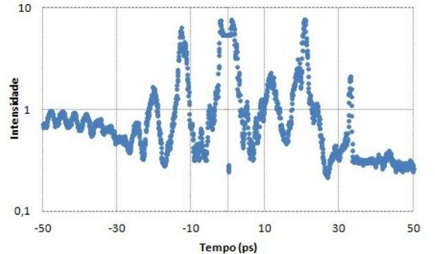
Figure 5: OPAC measurement over a 100 ps window.
