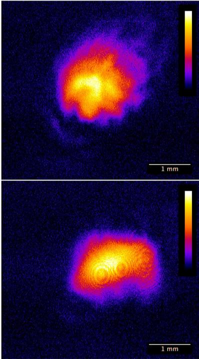
Figure 3: Signal (top) and idler (bottom) beams after the OPA crystal.
