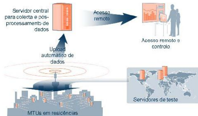
Figure 3 - System architecture used by ANACOM mobile tests, from [10]
