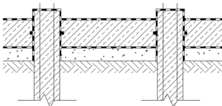
**Figure 6** - Scheme of the waterproofing system of a pile cap blocks [w<sub>3</sub>]
