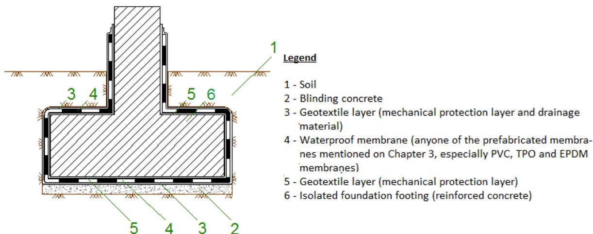
**Figure 2** – Waterproofing protection on an isolated foundation footing [personal archive]
