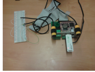
Fig. 7. Prototype of a node with short range infrared sensor capabilities.
