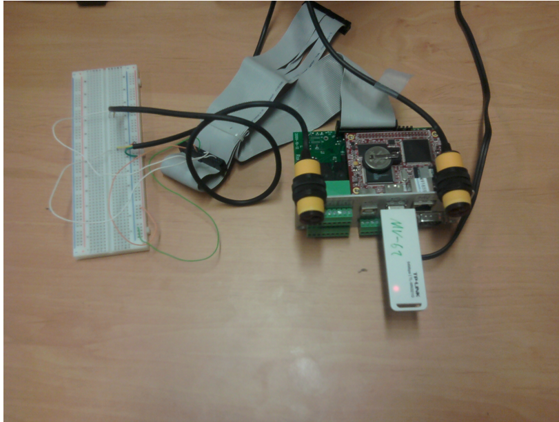
Figure 4.6: Prototype of a node with short range infrared sensor capabilities.
