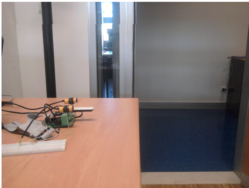
Figure 5.4: Node at the entrance of the inner division. Contains infra-red sensor and wi-fi USB dongle.
