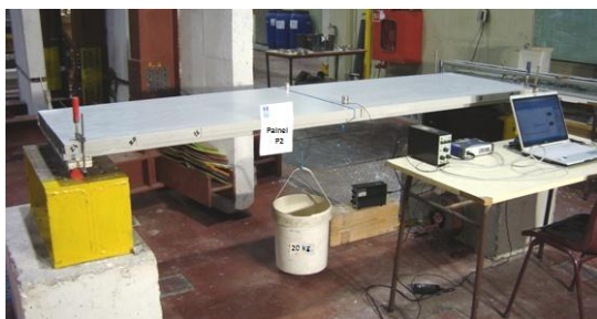
Figure 17 – Dynamic test setup.
