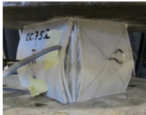
Figure 9 – Cell compressive test.
