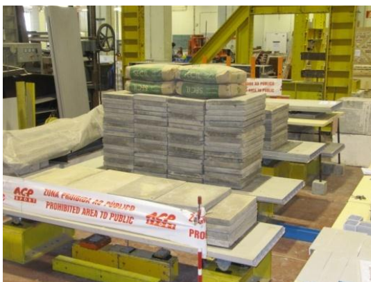
Figure 20 – Loading of panels for the creep test.
