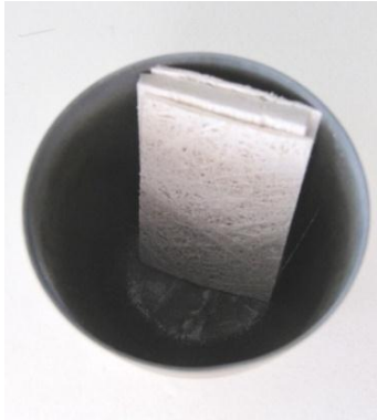
Figure 4 – Specimen after calcination.
