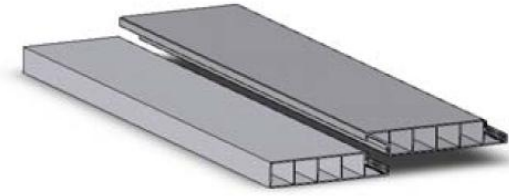
Figure 1 – Deck assembly by snap-fitting [2].
