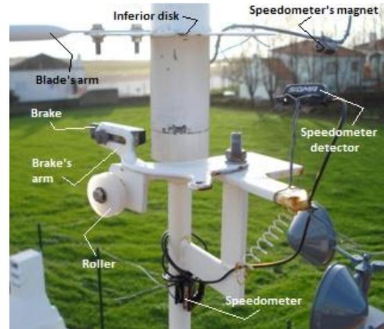
Figure 7 – Prototype detail
