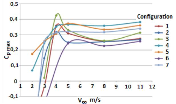
Graph 8 –  $C_{P_{\max}}$  according to  $V_\infty$  for all configurations
