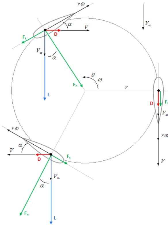
Figure 2 – VAWT's aerodynamic forces
