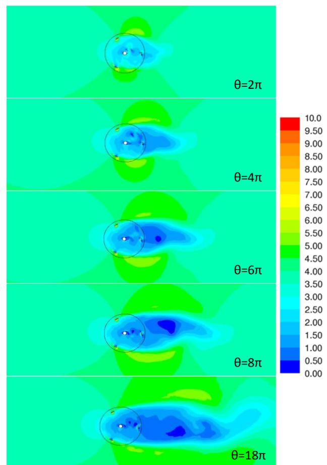
Figure 4 –  $|V|$  for configuration 5 with  $V_\infty=4m/s$ ,  $\lambda=4$
