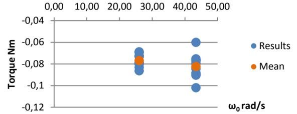
Graph 12 – Measurement 2 for the brake's calibration
