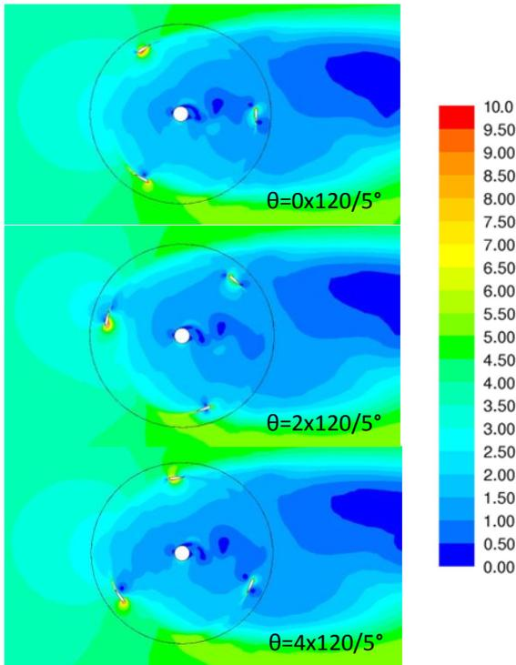
Figure 5 -  $|V|$  for configuration 5 with  $V_\infty=4\text{m/s}$ ,  $\lambda=4$  (detail at 4<sup>th</sup> turn)
