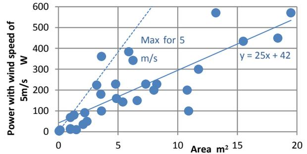
Graph 5 – Power produced at  $V_{\infty}=5$ m/s vs area
