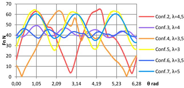
Graph 10 -  $|F_n|$  according to  $\theta$  for several configurations with  $V_\infty=8$  m/s and  $\lambda_{\text{optimum}}$ .
