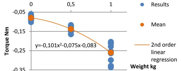
Graph 13 – Measurement 3 for the brake's calibration
