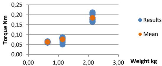
Graph 11 – Measurement 1 for the brake's calibration
