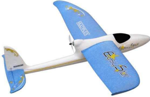
Fig. 4 Easystar UAV with 1.4m wingspan and 0.68kg of (empty) weight.
