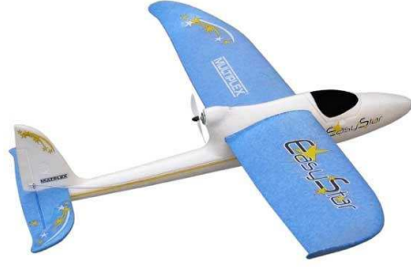
Figure 5.17: Easystar UAV with 1.4m wingspan and 0.68kg of (empty) weight.
