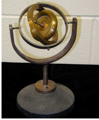
Figure 2.15: Conventional mechanical gyroscope (source: www.gyroscopes.org ).
