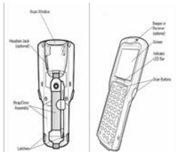
**Figure 4** Diagram of the scanner Symbol MC-3000
