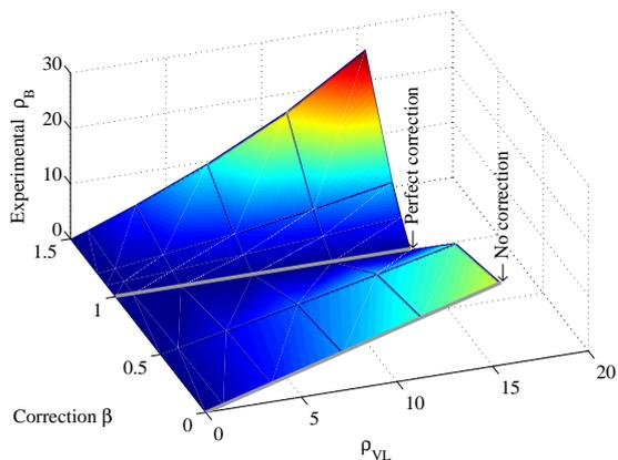
Fig. 3: Background standard deviation vs vignetting effects and corrections. The correction  $\beta$  is adimensional, while  $\rho_{VL}$  and  $\rho_B$  have their dimensions defined in a 8 bits gray-scale space.
