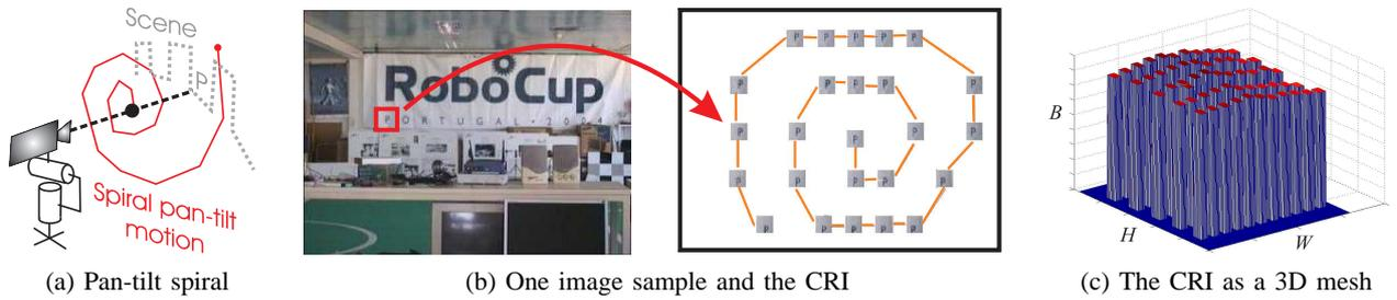
Fig. 2: Building a Constant Radiance Image (CRI). Camera motion (a) and sample (patch) collection (b). (c) Regular grid of patches, with brightness  $B$ , in a  $W \times H$  CRI, obtained with approx. constant pan-tilt steps (d).
