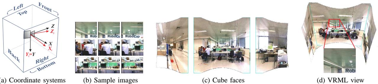
Fig. 1: Cube based background representation. (a) Coordinate systems of the cube,  $\{X, Y, Z\}$  and the pan-tilt camera,  $\{X_t, Y_t, Z_t\}$  with zero tilt and non-zero pan. (b) A number of the images captured to build a mosaic. (c) Left, front and right cube mosaicked-faces. (d) VRML view of the cube model showing one of the acquired images.
