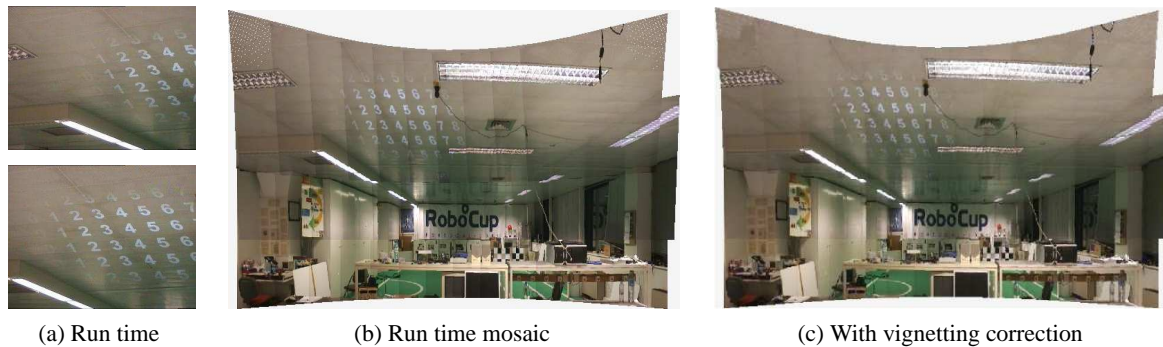
Figure 4.9: Run time view. Two run time images (a), a mosaic built from 47 run time images (b), and the same mosaic with vignetting correction (c).
