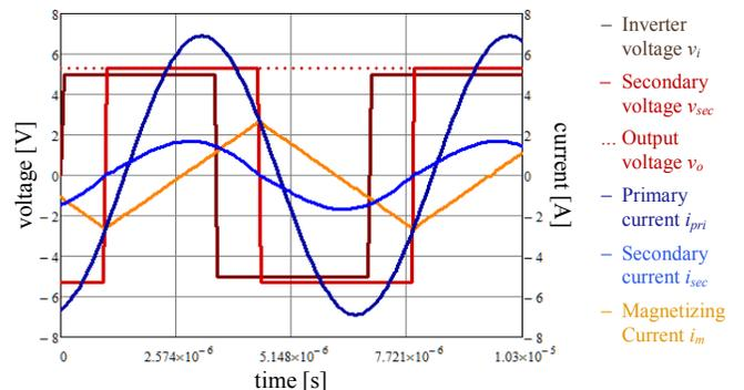
Fig. 6 – Simulation results of the resonant converter operating at full load
