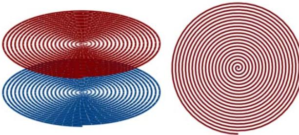
Fig. 1 – Coreless transformer windings configuration, used for contactless battery charging.
