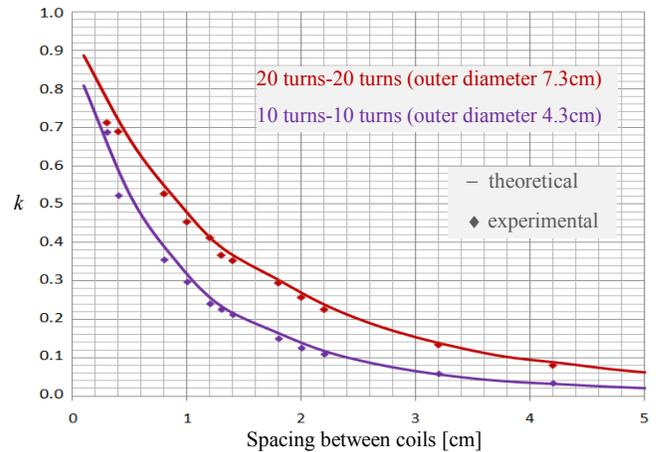
Fig. 3 – Magnetic coupling factor dependence with distance for concentric spiral coils.
