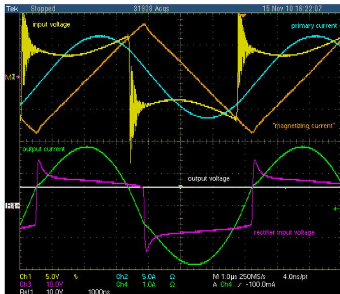
Fig. 7 – Experimental results with 20mm spacing and full-load operation. Ch1-Yellow trace → Inverter voltage; Ch2 - Blue trace → primary current; Ch3 - Magenta trace → Secondary voltage; Ch4 - Green trace → Secondary output current; Ref1 - White Trace → Output DC voltage.
