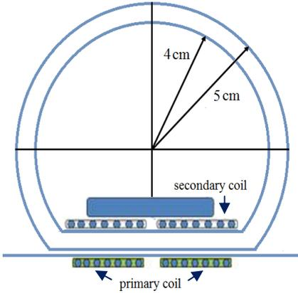
Fig. 2 – Structure of the spherical pack showing the receiver and transmitter spiral planar coils and their physical limitations.
