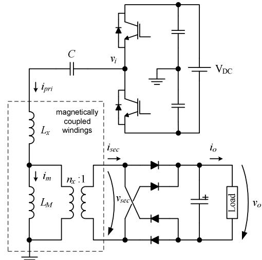
Fig. 5 – Resonant converter.
