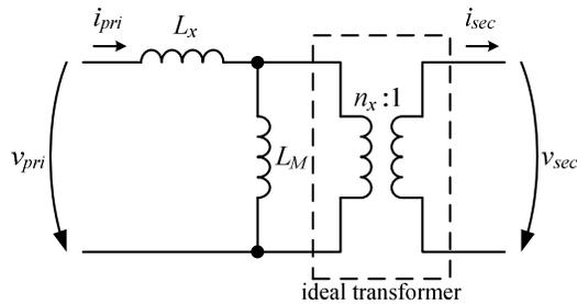
Fig. 4 – Equivalent three parameter transformer model.
