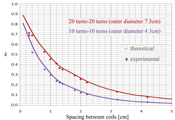
Fig. 3 – Magnetic coupling factor dependence with distance for concentric spiral coils.
