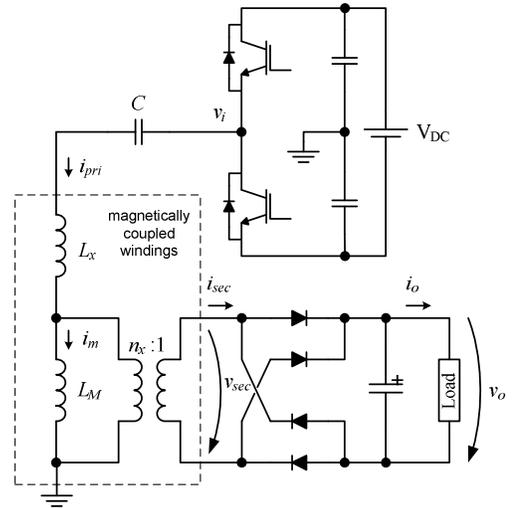
Fig. 5 – Resonant converter.
