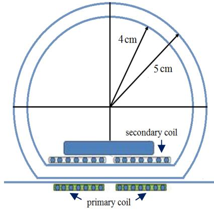
Fig. 2 – Structure of the spherical pack showing the receiver and transmitter planar coils and their physical limitations.
