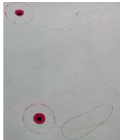
Figure 14: identification of cracks and craters in the weld [8]
