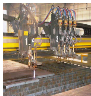
Figure 6: Details of implementation of plasma arc cutting and representative scheme of a plasma cutting torch with water injection [ph: personal archive] [3]
