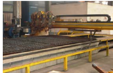
Figure 5: Equipment for oxy-fuel cutting [ph: personal archive]
