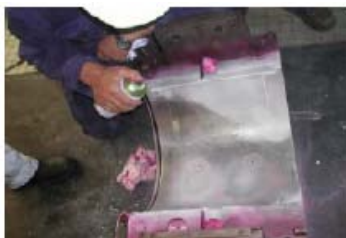
Figure 13: Liquid penetrant inspection [8]
