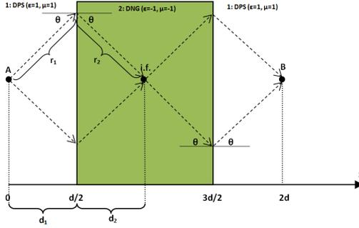
Figure 20. Passage of light waves through a Veselago flat lens, **A**: the image source, **B**: focused image, **i.f.**: the internal focus point
