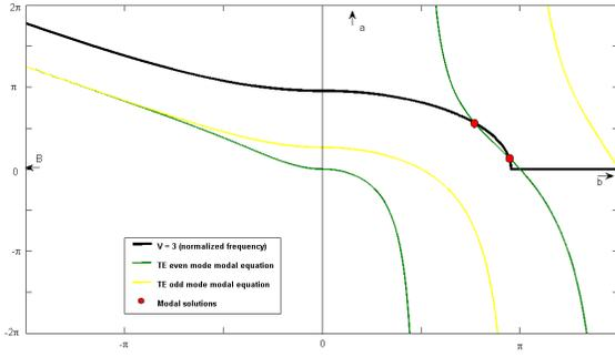
Figure 14. The representation of the modal solutions (red dots) given by the intersection of the curves for a DNG slab with  $\varepsilon_1 = \mu_1 = 1$ ,  $\varepsilon_2 = \mu_2 = -1.5$  and  $V = 3$
