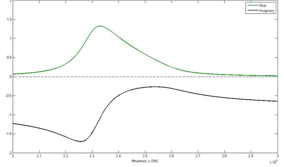
Figure 9. Attenuation constants  $\alpha_1$ , for the TM modes, using the lossy LDM, on the DPS-DNG interface
