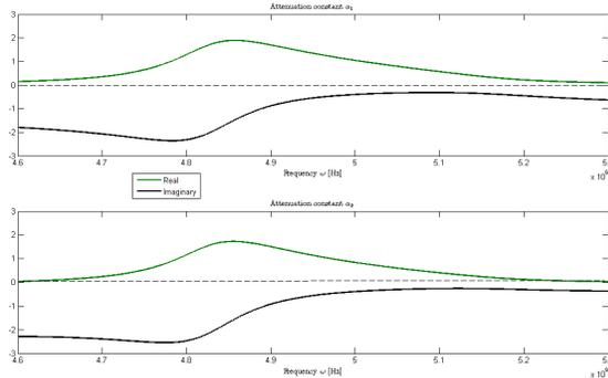
Figure 8. Attenuation constants  $\alpha_1$  and  $\alpha_2$ , for the TE modes, using the lossy LDM, on the DPS-DNG interface
