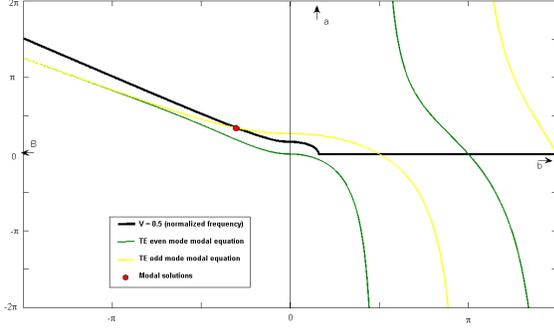
Figure 13. The representation of the modal solutions (red dots) given by the intersection of the curves for a DNG slab with  $\varepsilon_1 = \mu_1 = 1$ ,  $\varepsilon_2 = \mu_2 = -1.5$  and  $V = 0.5$
