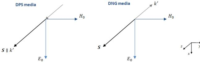
Figure 2. Spatial Representation of the fields, the energy flux and the propagation constant for a DPS and a DNG medium
