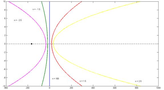
Figure 19. The lenses contours for different refraction indexes,  $n = -2.5, -1.5, 100, 1.5, 2.5$
