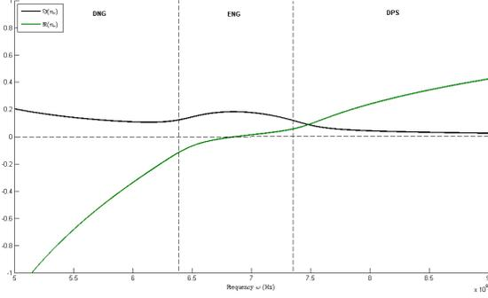
Figure 6. Relative refractive index ( $n_r = \frac{n}{\sqrt{\epsilon_0 \mu_0}}$ ), using the lossy LDM, on the DPS-DNG interface.
