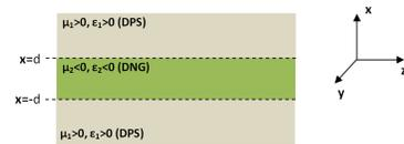
Figure 11. A DNG slab waveguide immersed on a DPS media
