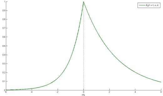
Figure 10. Variation of the electric field,  $E_y(t = 0, x, z)$ , on the DPS-DNG Interface
