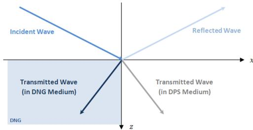
Figure 3. Scattering of a wave that incises on a DPS-DNG interface
