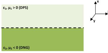
Figure 4. The planar interface between a DPS and a DNG medium, here represented by a dashed line.
