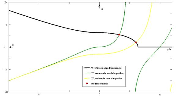
Figure 12. The representation of the modal solutions (red dots) given by the intersection of the curves for a DPS slab with  $\varepsilon_1 = \mu_1 = 1$  and  $\varepsilon_2 = \mu_2 = 2$ .
