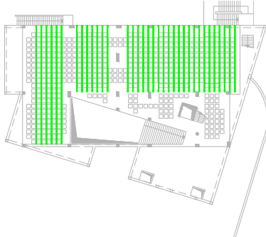
Image 16 – Pre-stressed strands distribution in 1st floor
