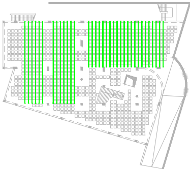
Image 15 – Pre-stressed strands distribution in ground floor
